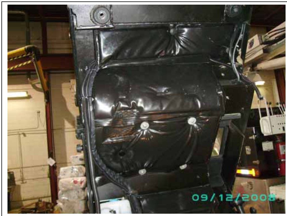
When install complete, tar tape fittings and hole at the evaporator.
