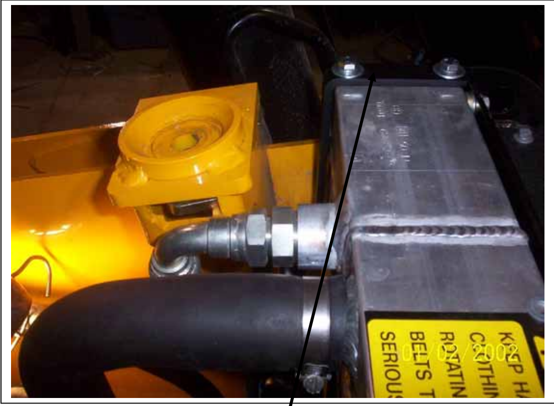
Install right hand upper condenser bracket as shown with hardware provided in kit.
