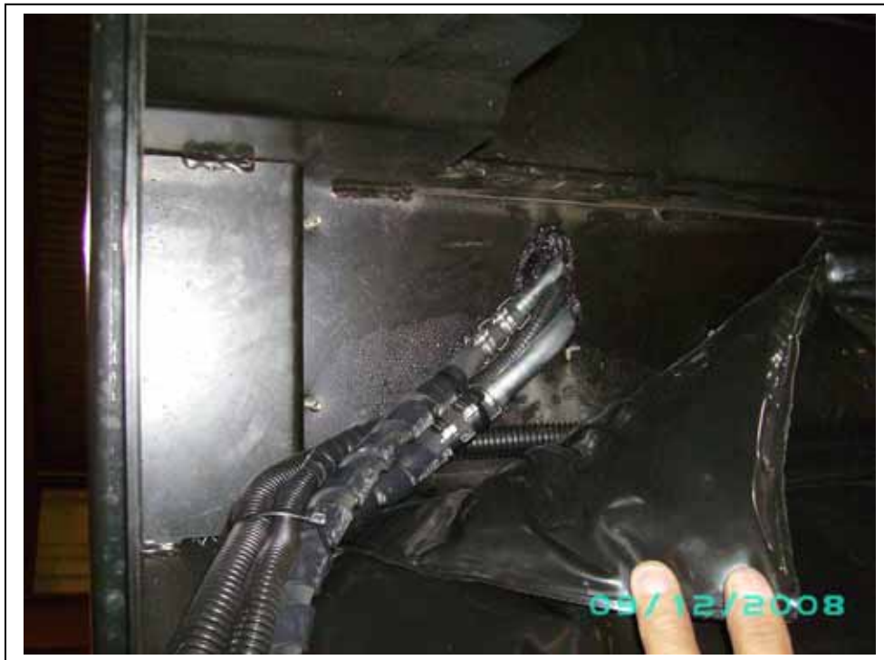
When install complete, tar tape fittings and hole at the evaporator.
