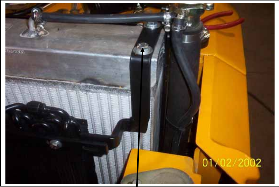
Left hand upper condenser bracket.
